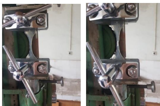
Figure 6. Formation of the neck at break
